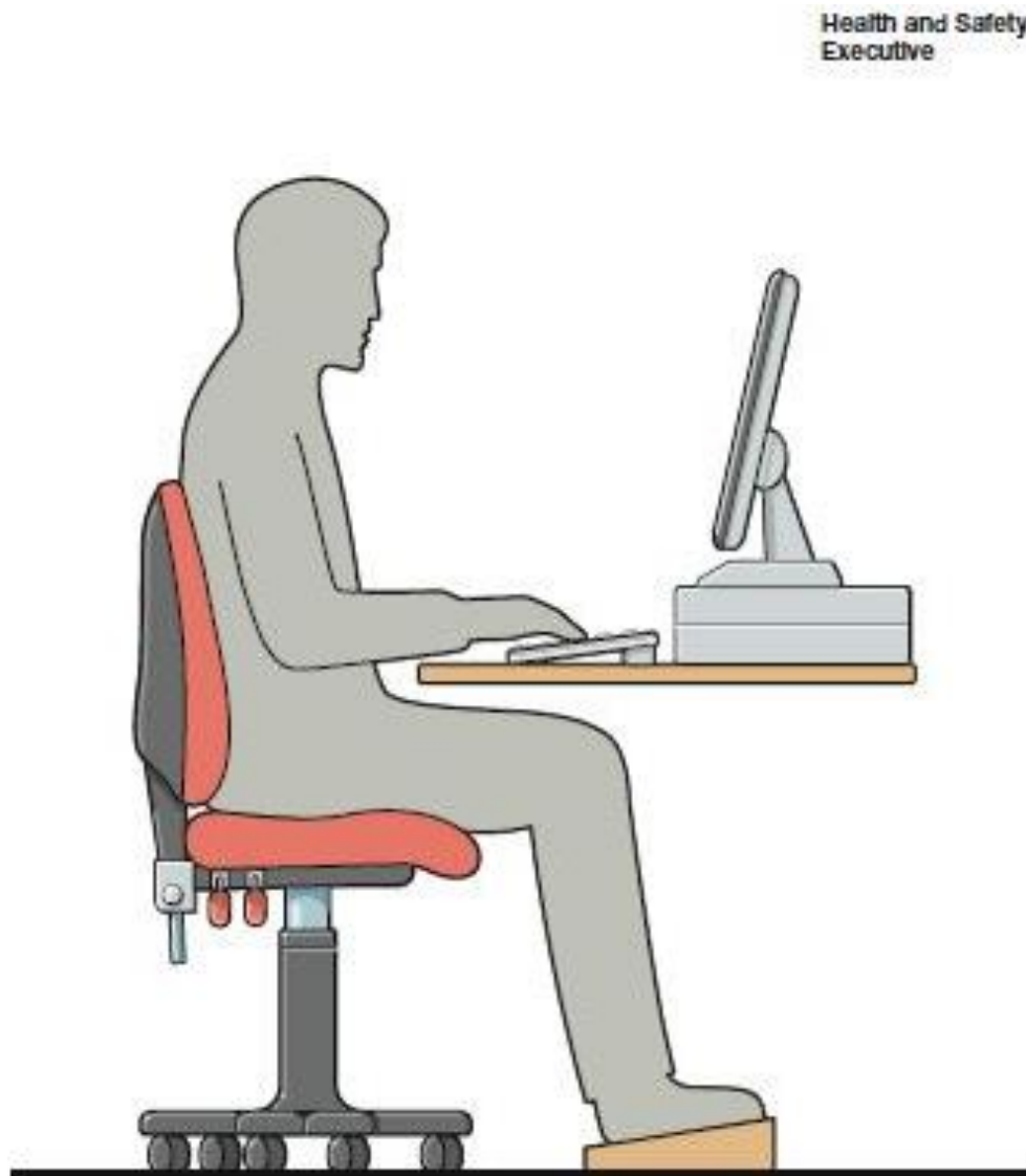
Figure 2 Seating and posture for typical office tasks
